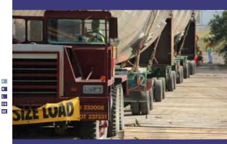
In order to keep this petrochemical plant's outage to just 28 days, Turner Industries completed pre-assembly of major process structures at an adjacent site during demolition of the existing equipment and piping.
