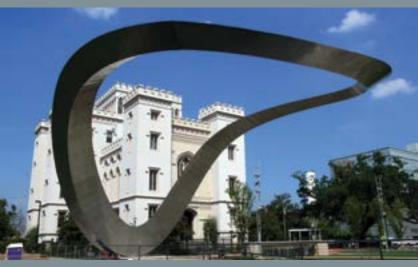
This 65,000-pound, 35-foot-tall steel cantilevered sculpture, which extends 85 feet and consists almost entirely of welded plates, serves as a final component of a city-wide revitalization effort in Baton Rouge.
