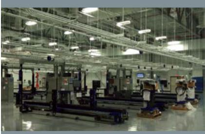
Brasfield & Gorrie constructed this \$32 million, 70,000-square-foot missile integration facility using "zero lift" technology, which relies on laser-guided vehicles to eliminate the risk of explosions.
