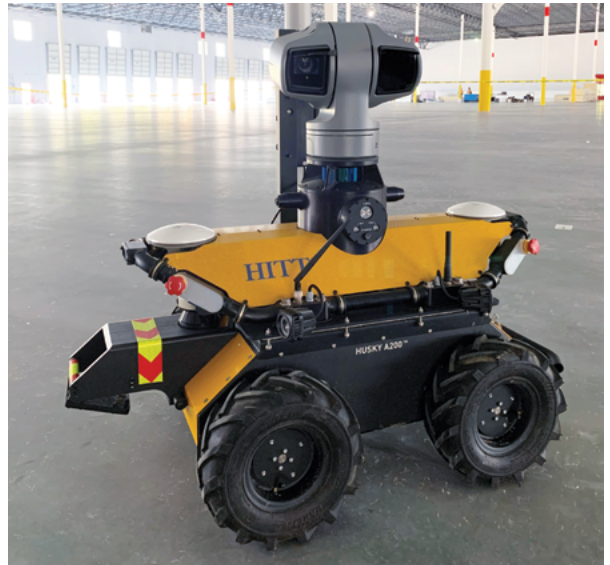
Figure 2. HITT's custom rover-style robot used for image capture, two-way communication
