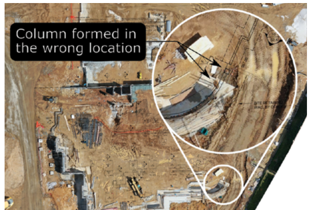
Figure 3. Quality control with drone imagery
