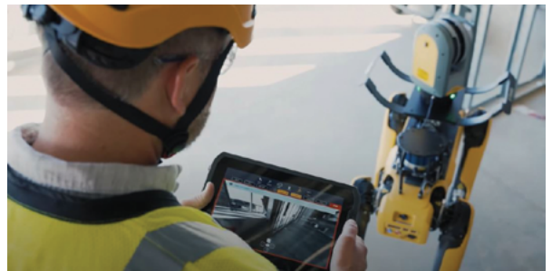
Figure 2. Robotics can help automate common tasks such as laser scanning or 3D photo documentation, increasing project staff efficiency
