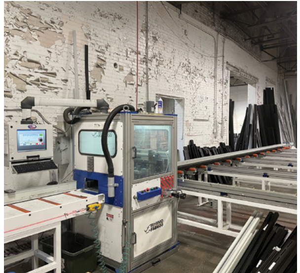
Figure 2. Fabrication center with 22-inch up-cut saw and three-axis drills for fabricating holes
