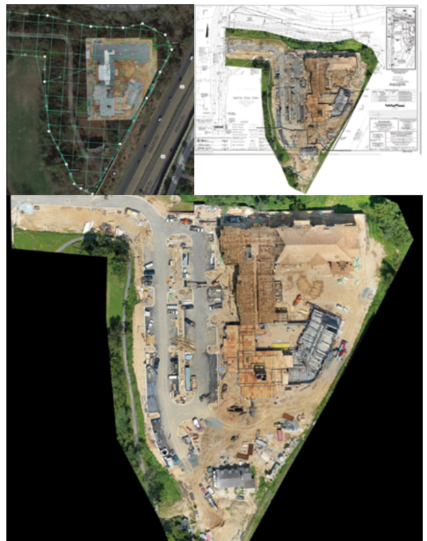
Figure 2. Flight planning, orthophoto and drawing overlay
